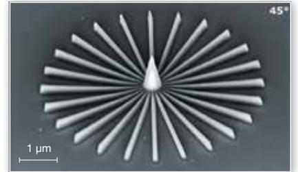
*Electron-beam-induced deposition for a star-like test pattern of silicon oxide.*
