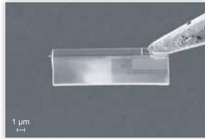
With the help of a nano manipulator, the pre-thinned lamella is transferred to a dedicated sample holder such as a TEM grid.
