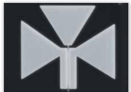
Demo example (transistor like pattern) showing EBL overlay capabilities.
