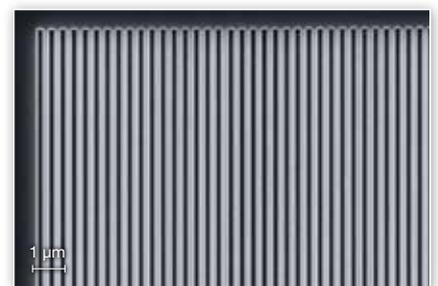
Placement, straightness and pitch of the 3-dimensional grating are checked by SEM inspection.
