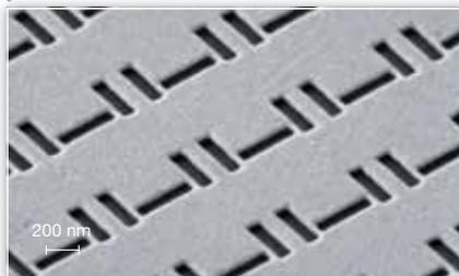
Stable and automated FIB milling enables large arrays of high-resolution features, as required for plasmonic applications.
