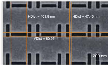
Detailed in-situ SEM inspection of plasmonic features created by FIB milling.
