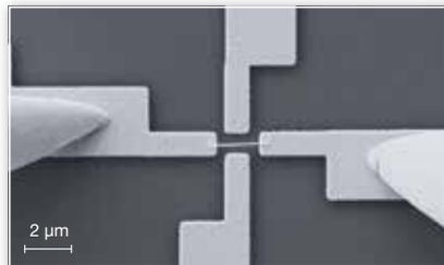
*Tungsten deposit between prefabricated gold contacts used for electrical conductivity measurements with nano probers.*
