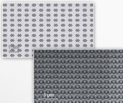
Direct FIB milling for high resolution (1) or 3-dimensional structures (2).
