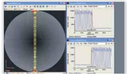
The roundness of an X-ray lens is checked by advanced SEM metrology line scans.
