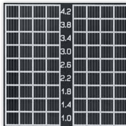
EBL test pattern for determining the line width for different dose factors.
