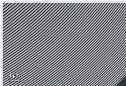
Top-down high-resolution SEM imaging used for lateral process control of FIB milling results.
