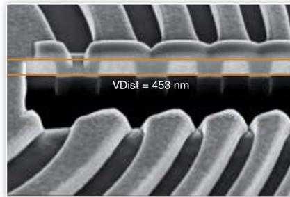
X-sectional process control of an X-ray Fresnel zone plate fabricated in 500 nm thick gold.
