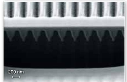
The 3-dimensional shape of a special antireflective grating is revealed by X-section analysis.
