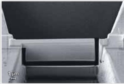
After deposition of a protective layer, a TEM lamella is cut out of the bulk sample at a specific site.
