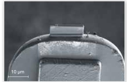
Once the lamella is connected to the TEM grid it is polished to the desired thickness, providing electron transparency.
